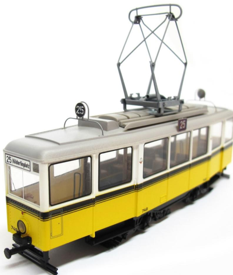
*The KSW or war tramcar was designed as a replacement for wagons destroyed in World War II: material-saving lightweight construction, easy to maintain, and with plenty of standing room and thus a high number of passengers. Around 700 of the mostly wooden wagons were delivered to over 20 cities, including Stuttgart, Munich and Cologne, between 1943 and 1950.*
