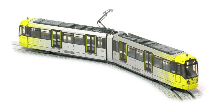
The **M5000 from Alstom** (formerly Bombardier) is a light rail vehicle. It belongs to the Flexity Swift series, which was specially built as a high-floor articulated streetcar for exclusive use on the Metrolink system in Manchester, England. It is a great honor for the small Viennese model railroad manufacturer HALLING Modelle to be able to realize this very successful prototype in a model!
